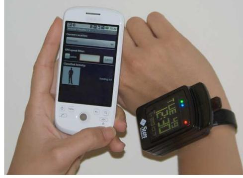
Figure 3. COSAR implementation for Android and smart watch prototype
